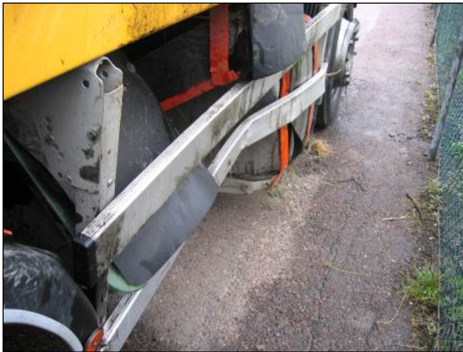
Figure 56 Rear and Side Underrun Protection deformation detail
