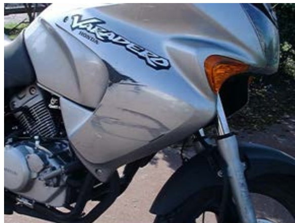
Figure 68 Typical PTW side body, gas tank and front forks damage
