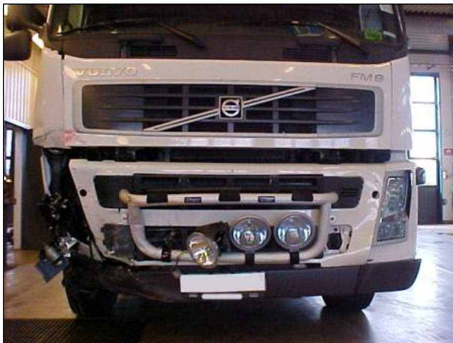
Figure 54 Frontal Underrun Protection deformation detail
