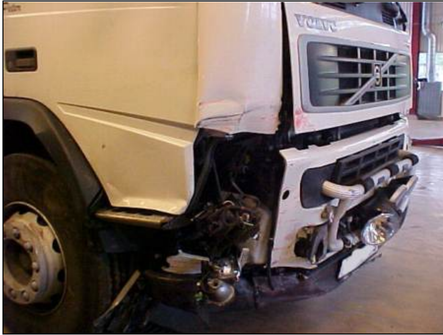
Figure 55 Frontal Underrun Protection deformation detail
