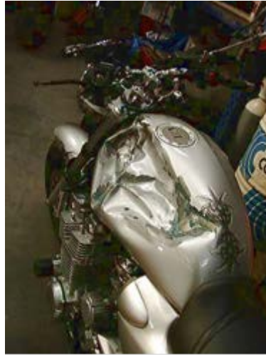
Figure 69 Typical PTW side body, gas tank and front forks damage
