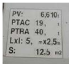
Figure 96 Specifications plate (values from top to bottom: vehicle weight with no load, gross vehicle weight rating, authorised gross vehicle weight, length and width measurements (respectively), surface area)
