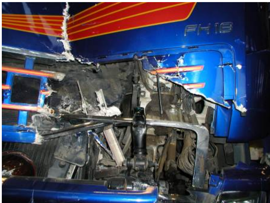
Figure 58 Cabin displacement detail
