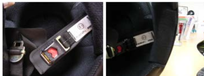
Figure 78 PTW Helmet (note the fastener detail)
