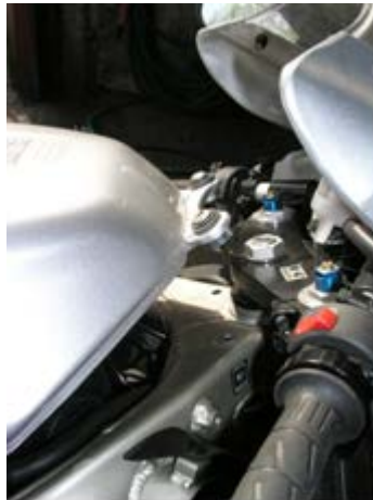
Figure 67 Typical PTW side body, gas tank and front forks damage
