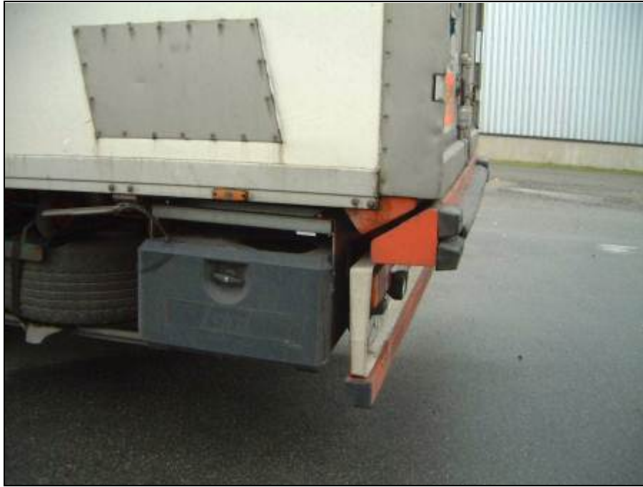
Figure 57 Rear and Side Underrun Protection deformation detail
