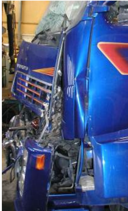
Figure 59 Cabin displacement detail
