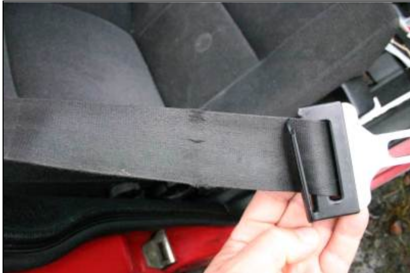
Figure 34 Seatbelt detail photo (note the damage to the belt)
